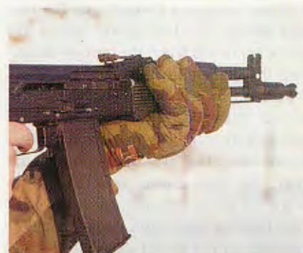
AK105, chambered for the 5.45x39mm round, has a 12.4-inch barrel with an effective muzzle device and a side-folding buttstock.
